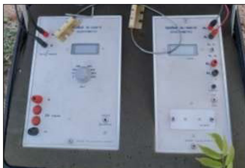
Figura 7: Resistivímetro, Geotest RD-1000A
